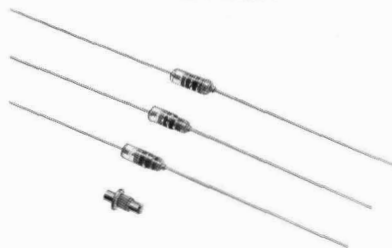
Fig. 3. Step Recovery Diodes in glass and ceramic packages. Ceramic package is designed to be especially useful with coaxial structures but can also be used in other ways as in Fig. 8.
